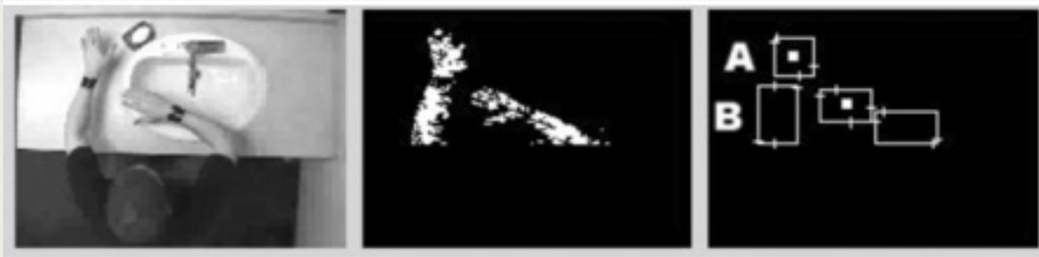
Determining the hand's location given two vertically stacked blobs.
